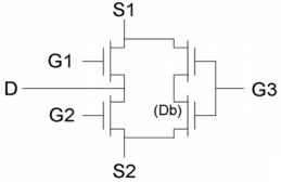
Both of the synchronous rectifier MOSFETs share the common drain connection D, but their sources S1 and S2 and gates G1 and G2 are separate. If the sources are interdigitated, with a pitch P that is small compared to the die thickness L, the area of the drain D is shared and the current density at the drain is halved. High frequency effects are minimized.
