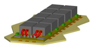
The components of the SCPC could be directly installed on the motherboard, but there are advantages to using a separate daughterboard. All of the fine pitch connections for the solder bumps are confined to the small daughter board, and the entire circuit can be tested before assembly.
