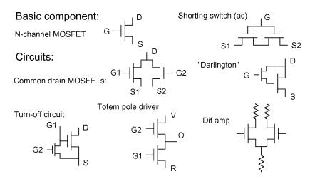
With resistors, many more circuits based upon the old RTL integrated circuit logic family (from the 1960's) can be made, by substituting n-channel MOSFETs for the NPN bipolar transistors.
