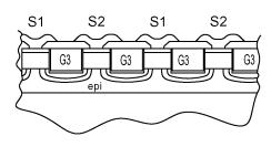
In the schematic, the shorting switch looks like two devices, two MOSFETs back to back, functionally, and it must block current in either direction when off. In the power IC, the shorting switch is implemented using single trenches with a common gate G3. The sources S1 and S2 are interdigitated alternately on opposite sides of adjacent trenches. No separate terminations
