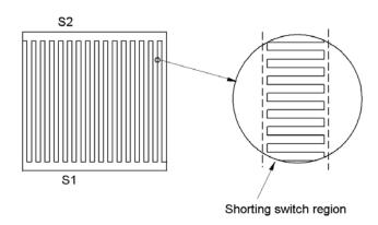
require no connection. However, they must be isolated from the other circuits, so there is an isolation barrier under the area occupied by the shorting switch.
