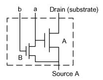
on the MOSFET A is much less critical, so it is turned on conventionally with a signal applied to its gate a by the high side driver located in the logic IC.
