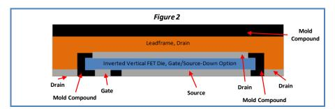
Figure 3: Rugged leadframe structure showing inverted vertical power FET die in bottom-side leadframe cavity with drain connected to leadframe, which can be clamped between top & bottom cold plates for high power dissipation in applications like EV/HEV.
