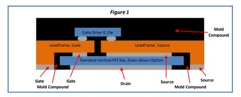
Figure 2: μMaxPak Single-Switch Cross-section showing inverted vertical power FET die in bottom-side leadframe cavity with drain connected to leadframe.
